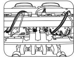
4. Turn off both dip switches pin no. 2 of the display PCB on the button display panel and pin no. 2 of the main PCB inside.
