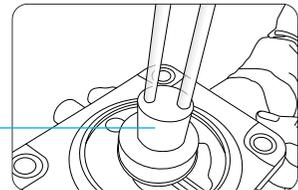
6. Fasten the two pairs of dasher cover bolts facing each other diagonally.
