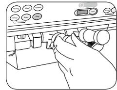
3. By taking out the button display panel on the bottom and turning it upside down, you can place it on top of the product. At this time, do not damage the PCB wire and connectors.
