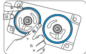
5. Insert the mixing shaft and align the dasher bearing.
