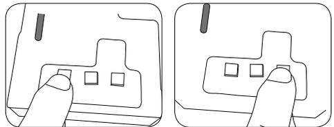
11. When the downloading is completed, remove the downloading connector and turn on all the pins of the 2 pin dip switch.
