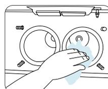
9. Remove the dasher brush and clean the blade hole with a brush and wipe out moisture with a soft cloth.
