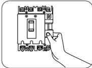
⚠ Install it independently with an earth leakage circuit breaker with more than 50[A].
