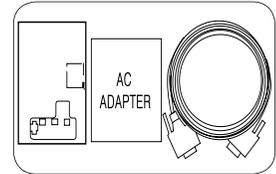
2. Connect the RS-232C cable to the serial port of the PC and plug the AC power adapter into a power outlet
