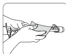
11. Extract a handle shaft and separate the lever from the dasher cover.
