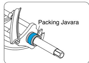
4. Insert the dasher assembly into the cylinder.
