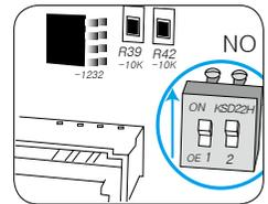
9. Prepare a download kit with the latest version of the program. Insert it into the download connector (left to the dip switch) of the main PCB.
