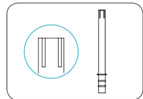
This figure shows the caburator aligned with a large hole. Align the large hole of the upper area of the caburator body with the large hole in the upper area of the tube. Decrease the overrun and increase the amount of ingredients injection in this way when you need continuous vending of the product. Condition of use: When the "AUTO" mode is executed
