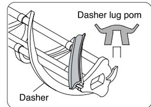
2. Apply food grade grease on the shaft and insert it into the dasher.
