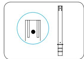
This figure shows the caburator aligned with a medium hole. Align the medium hole of the upper area of the caburator body with the medium hole in the upper area of the tube. Then, it will be aligned with the medium hole in the lower area of the caburator body. It will make the overrun and the amount of ingredients injection at medium level for sales Condition of use: When the "AUTO" mode is executed
