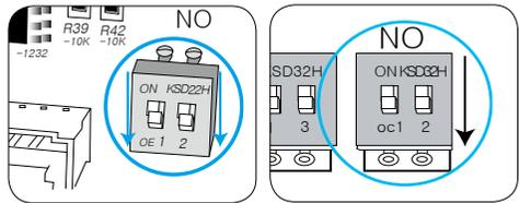
5. Prepare a download kit with the latest version of program. Insert it into the download connector (left of the dip switch) for the main PCB.
