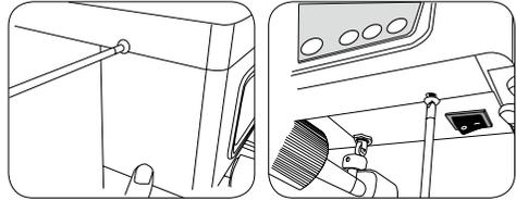
2. While pulling out the lever shaft, separate the sales lever. At this time, please be careful not to drop the sales lever. It can easily get damaged.
