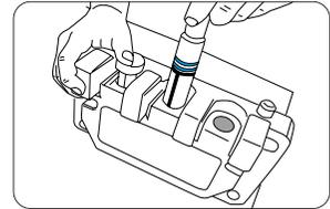
3. Insert the discharge lever into the piston and then insert the lever in line with the dasher cover and the discharge lever.
