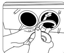
8. Brush off the inner area of the cylinder and wipe it off with a soft cloth.
