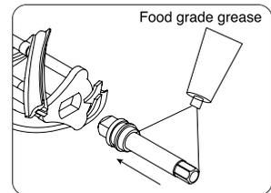
3. Check the direction of the packing javara and push it as deep as possible to prevent from coming off.
