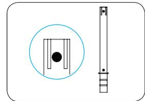
This figure shows the caburator aligned with a small hole. Align the small hole of the upper area of the caburator body with the small hole in the upper area of the tube. Then, it will be aligned with the small hole in the lower area of the caburator body. Increase the overrun and decrease the amount of ingredients injection in this way when you expect a small amount of sales. Condition of use: When the "AUTO" mode is executed
