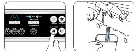
6. Stop the product by pressing wash button (do not turn off the power switch) and loose the dasher cover bolts diagonally by the order shown in the picture and separate the dasher cover from the machine.
