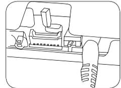
4. Connect the RS-232C cable to the download kit and run the download software.
