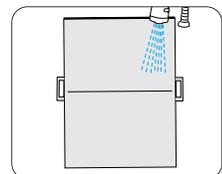
3. The condenser surface has lots of dust. Remove it by using a household vacuum cleaner or hand held cleaner. Clean and dry the filter and insert it into the machine.
