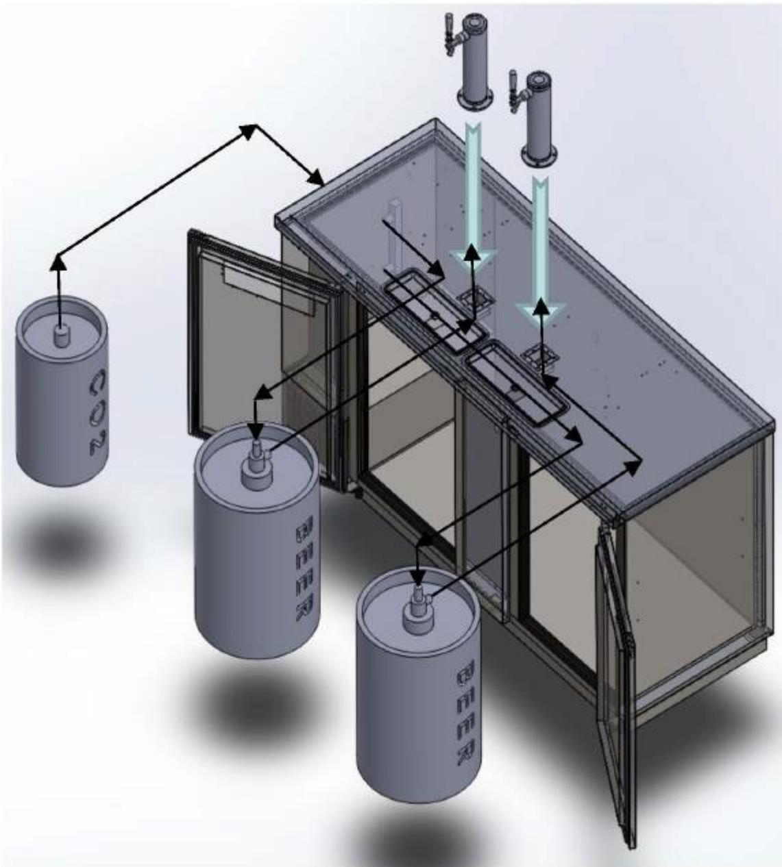
※ Assemble Beer Line & CO<sub>2</sub> Line as above drawing.
