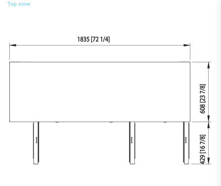
3 Doors Capacity 19.6 Cu.Ft. **Shelves** 6 Refrigerant R-290 **Temperature** 33°F ~ 39°F Range Easy Sliding Maintenance **Condensing Unit** 9.8 ft long (3m) flexible three Connection wire cord with modeled plug HP 3/8 Voltage 115V/60Hz **Amps** 3.5 **NEMA Config.** NEMA 5-15 Lighting Interior LED lighting
