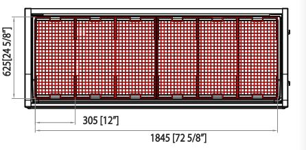
Basket 6 Capacity 24.72 Cu.Ft. Doors 2 Refrigerant R-290 -10°F ~ 0°F Easy Sliding Maintenance **Condensing Unit** 9.8 ft long (3m) flexible three Connection wire cord with modeled plug HP 3/4 Voltage 115V/60Hz **Amps** 3.8 **NEMA Config.** NEMA 5-20 Lighting Interior LED lighting
